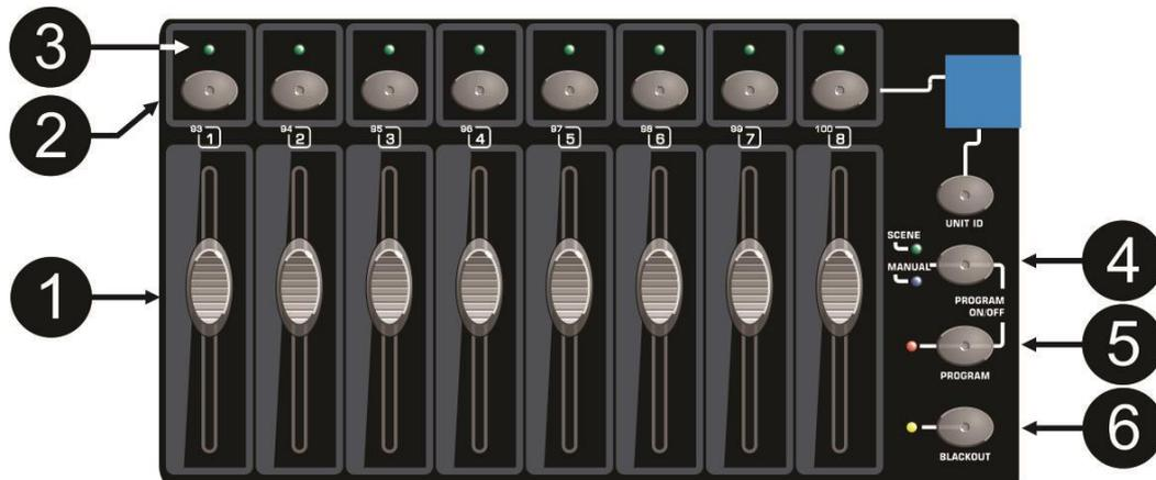
1. **CHANNEL FADERS:** can be used for different purposes, depending on the working mode:
