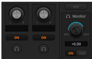
The monitor volume knob and buttons set independent audio levels and allow solo monitoring on the monitor XLR output
