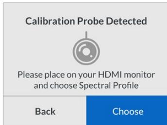
3.10 If your probe has a protective cover, remove it. Place the calibration probe in front of the monitor with the opening of the probe's sensor parallel to the screen and gently touching the middle of the white square displayed in the center of the screen.
