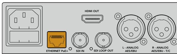
Connect power to your Teranex Mini converter using a standard IEC power cable. Power can also be supplied via a PoE+ compatible Ethernet switch.
