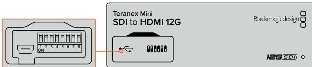
Change settings by adjusting the switches with a pen.
