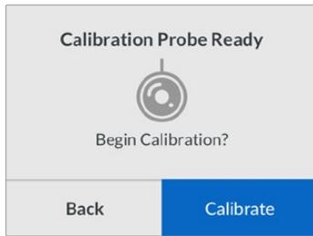
3.15 The calibration process takes 10-15 minutes. Teranex Mini SDI to DisplayPort 8K HDR generates and measures a wide range of colors at varying luminance values, comparing the measured results against the expected values. When the procedure concludes, it generates a calibration 3D LUT and shows a confirmation message.
