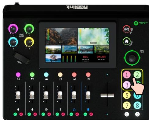
3. Use the Adjuster on the front panel for zoom-in and zoom-out of Layer A and the Joystick to quickly adjust horizontal and vertical position. Push joystick to full screen mode, then push it again to restore to the size and position last set.
