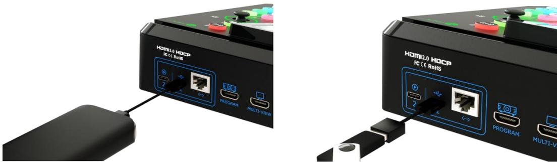
Insert a U disk or SSD to USB port labeled number 1. Before recording, format the U-disk or SSD first.
