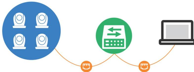
4) Connect mini-mx and camera to the switch via Ethernet cables (It is recommended to use RGBlink CAT6 cable with order code as 940-0001-00-11-0). Then use mini-mx for PTZ control.
