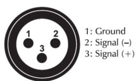
DMX-input XLR mounting-plug:
