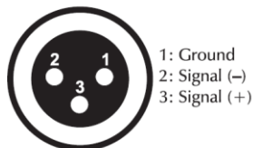
DMX-output XLR mounting-socket:
