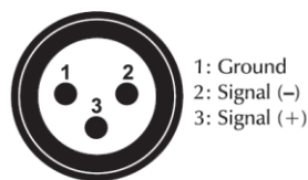
DMX-input XLR mounting-plug:
