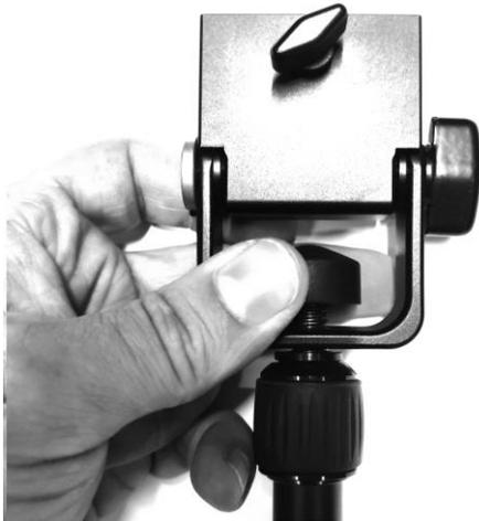
6. Insert the 50/50 glass beam splitter (Item F) into the Adjustable beam splitter glass clamp (Item D), the glass should be in landscape orientation as shown. Turn the thumb screw clockwise to secure the glass. The glass should be angled at approximately 40 degrees. You should be able to see the entire 15" LCD screen in the glass when stood directly in front of the teleprompter.
