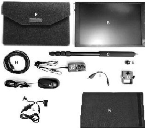
2. Lift out the 15" LCD control unit (Item B) and remove all other items in the case.
