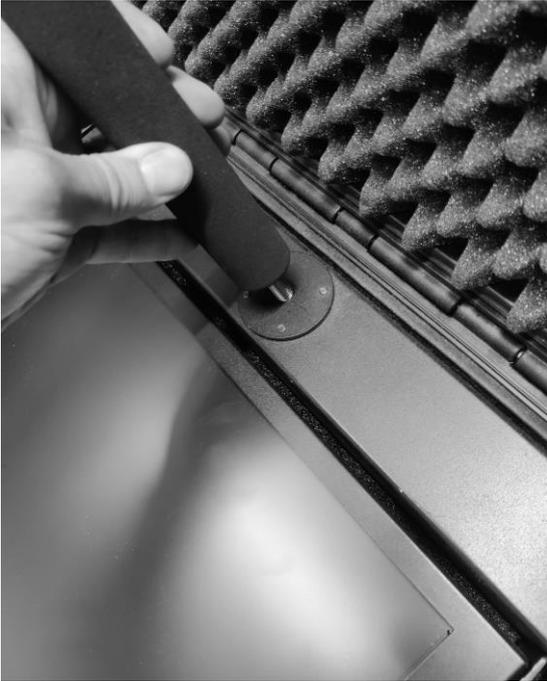
5. Attach the Adjustable beam splitter glass clamp (Item D) to the top of the extendable pole (Item C) using the thumb screw (Item E)
