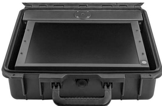
3. Put the 15" LCD control unit (Item B) back into the main TP-800 ENG hard case & chassis (Item A).
